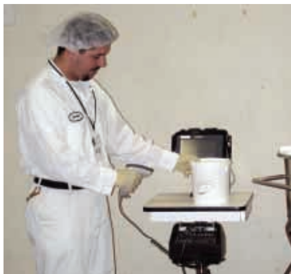
Operators simply scan a bar code label on the raw material ingredient container to verify that the correct ingredient and lot have been selected.
